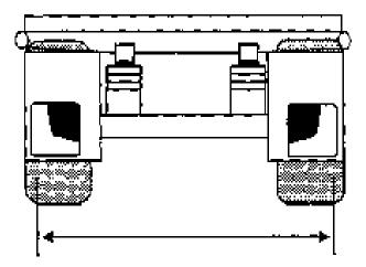
Illustration of overall axle ground contact width
