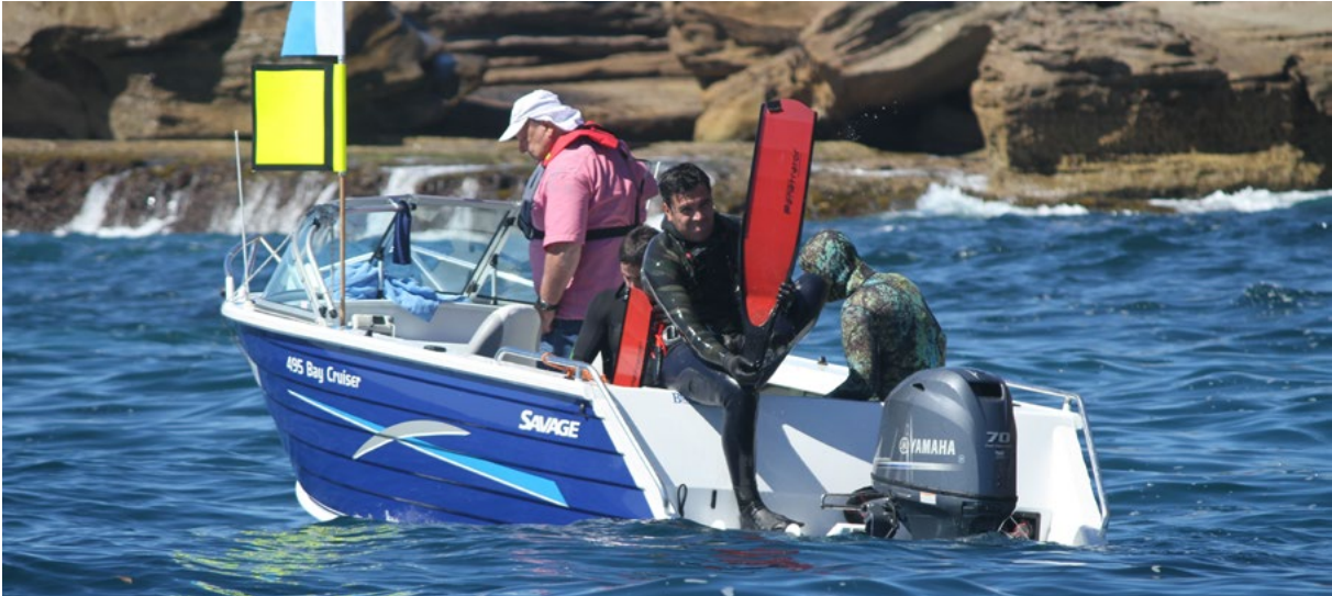
When divers or snorkellers are operating from a vessel, the blue and white alpha flag must be displayed, and a hi-viz addition is a good idea.
