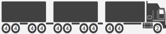
Rigid Truck and Two Dog Trailer Combination Length: 36.5 metres
