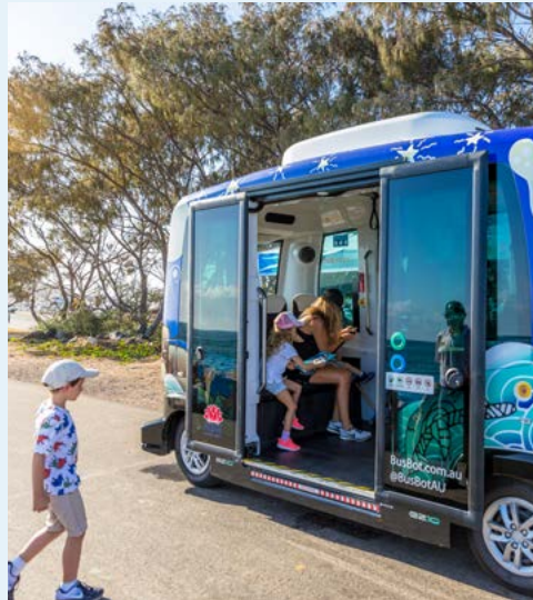
In an Australian first, the driverless BusBot was trialled in Coffs Harbour. This Level 4, fully automated EZ10 vehicle can carry up to 14 passengers.
