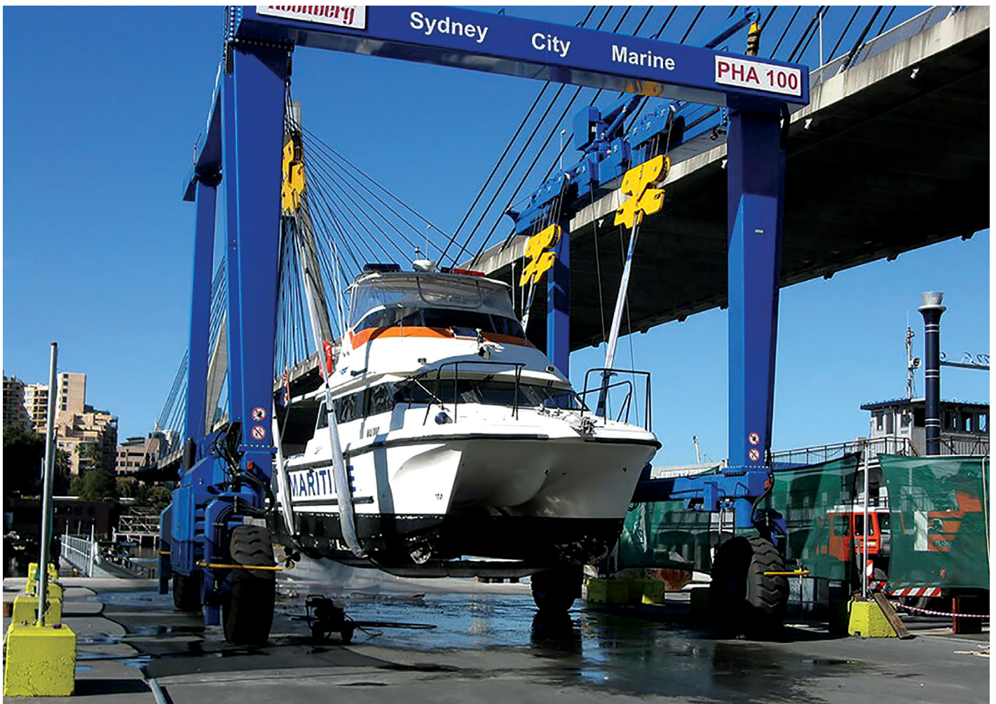
Example of a boat travel lift. Image supplied by Sydney City Marine
