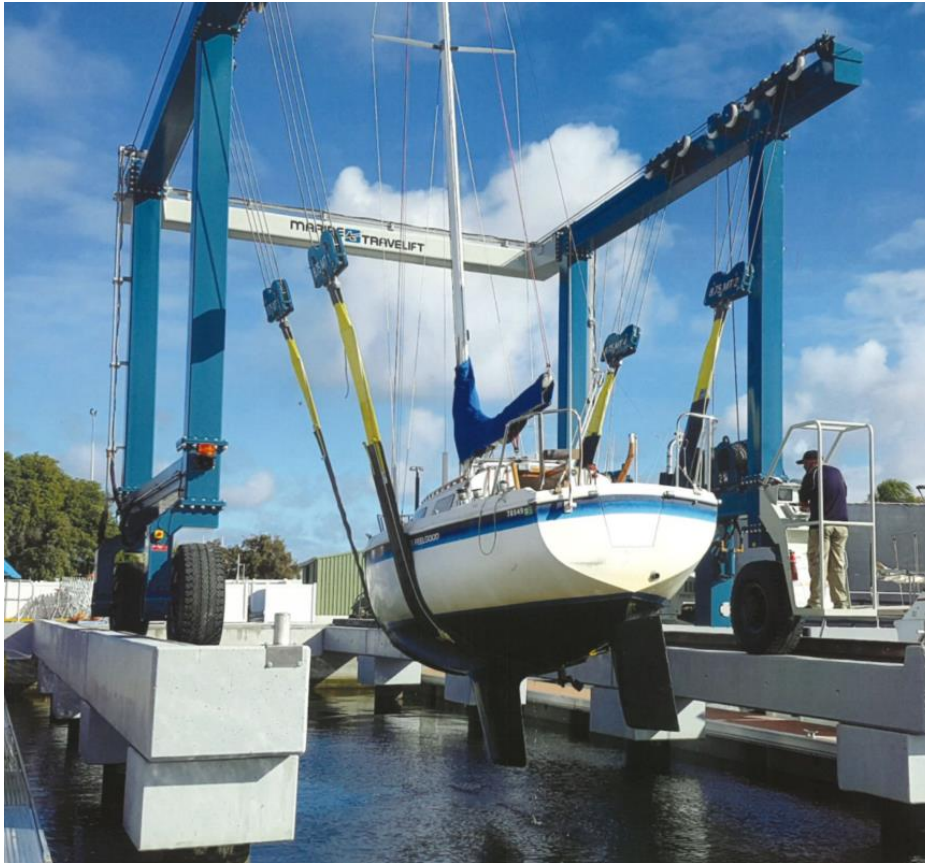
Figure 19: Example travel lift facility (Source: Waterline cover page 2020-2nd quarter, Marine Industries Association)
