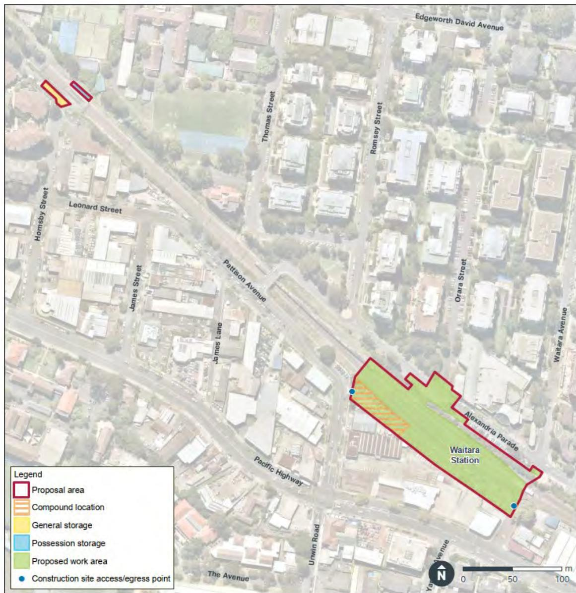
**Figure 1-3 Work areas and compound locations required for the Proposed Activity as displayed in the REF (indicative only, subject to detailed design)**
