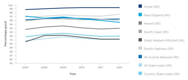
Note: Measurements for Figure 8 according to International Roughness Index (IRI).
