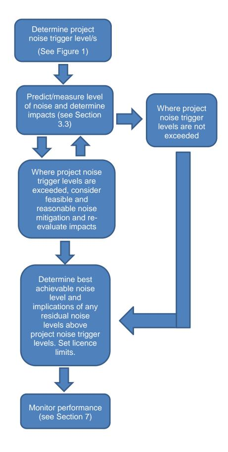
Figure 2: Typical noise impact assessment process.
