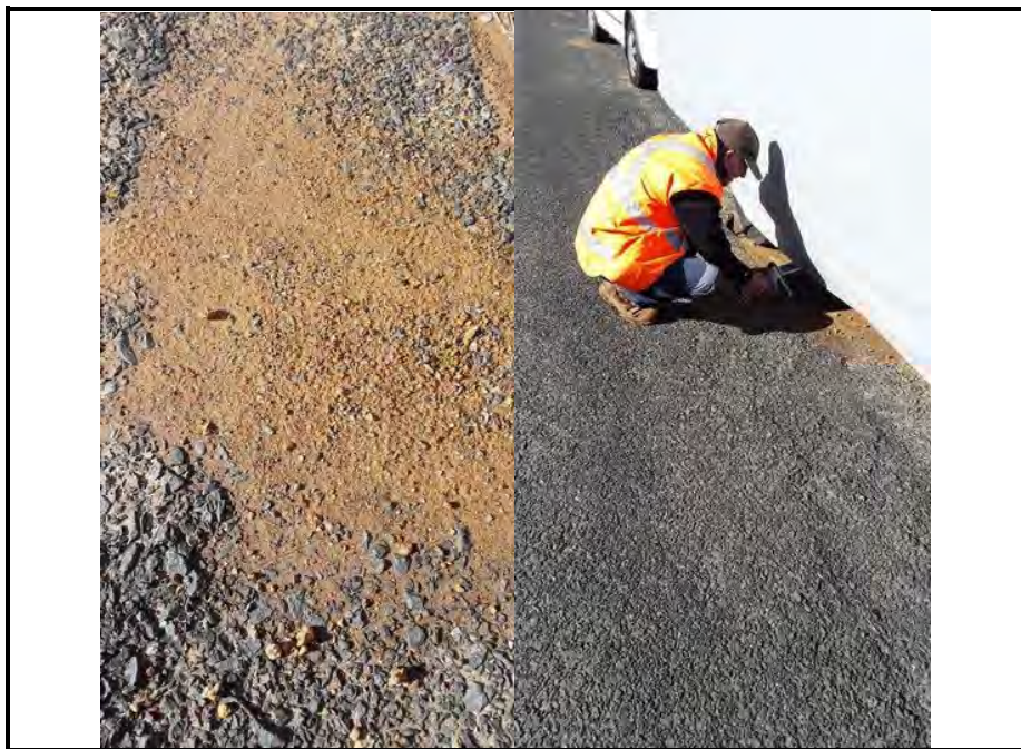
Photo 20: Photograph of the sediment sample DS01 build up on road of Ottiwell St and XRF testing of the sediment
