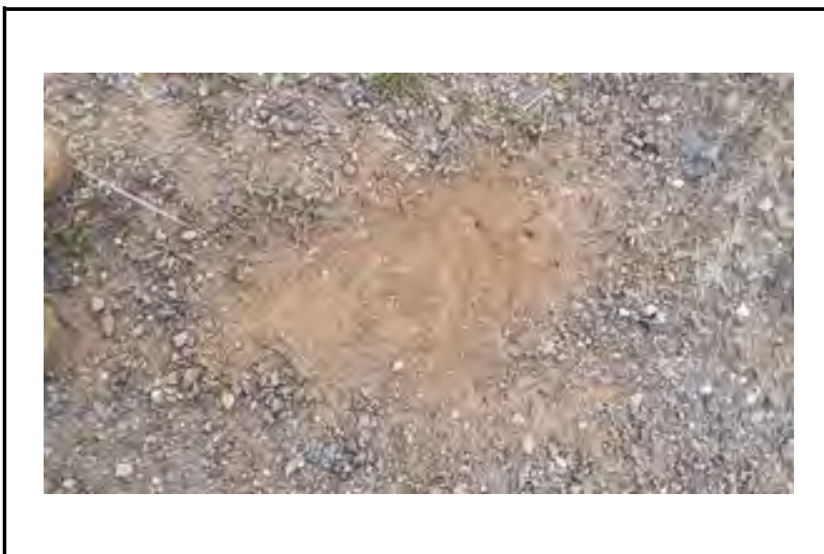
Photo 4: Brown gravelly silt. High percentage of gravel within this area with grass mostly constricted to fence line. Heavy vehicle traffic within this area. Sample XS010
