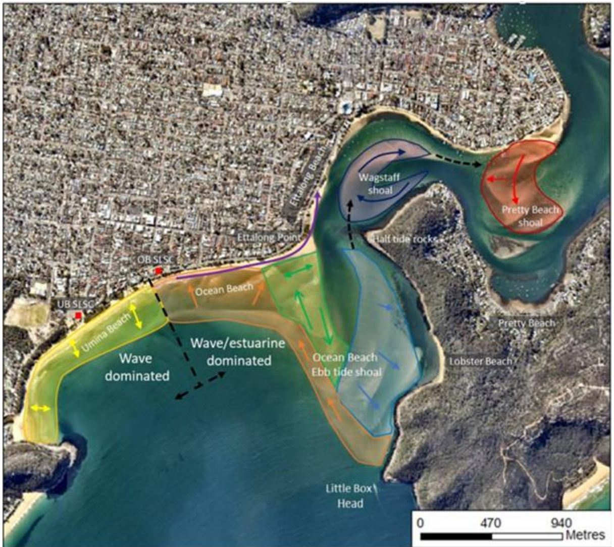
Figure 3-1: Ocean Beach - Ettalong Beach conceptual sediment transport model. Source: WRL, 2021.
