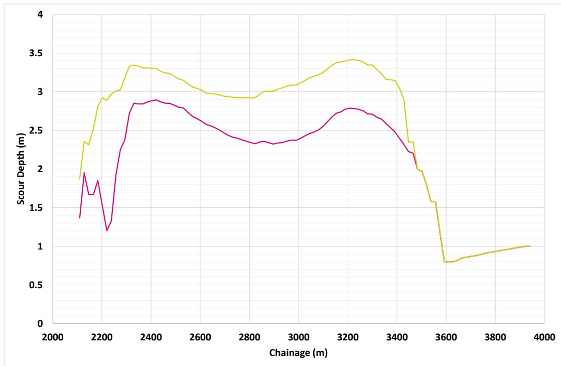
Figure 4-6 Estimated Scour Depth at BR021
