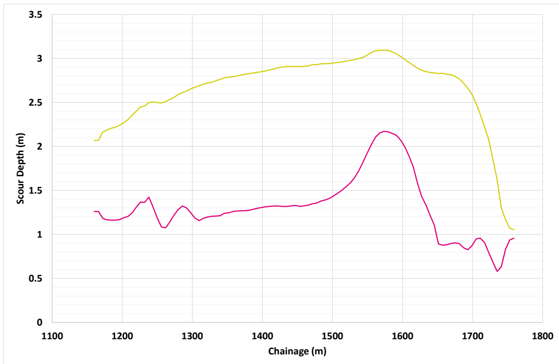
Figure 4-3 Estimated Scour Depth at BR011
