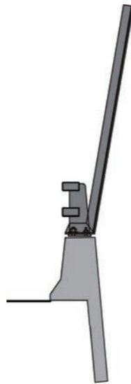
Figure 81: Detailed Profile of Throw Screen Type 1
