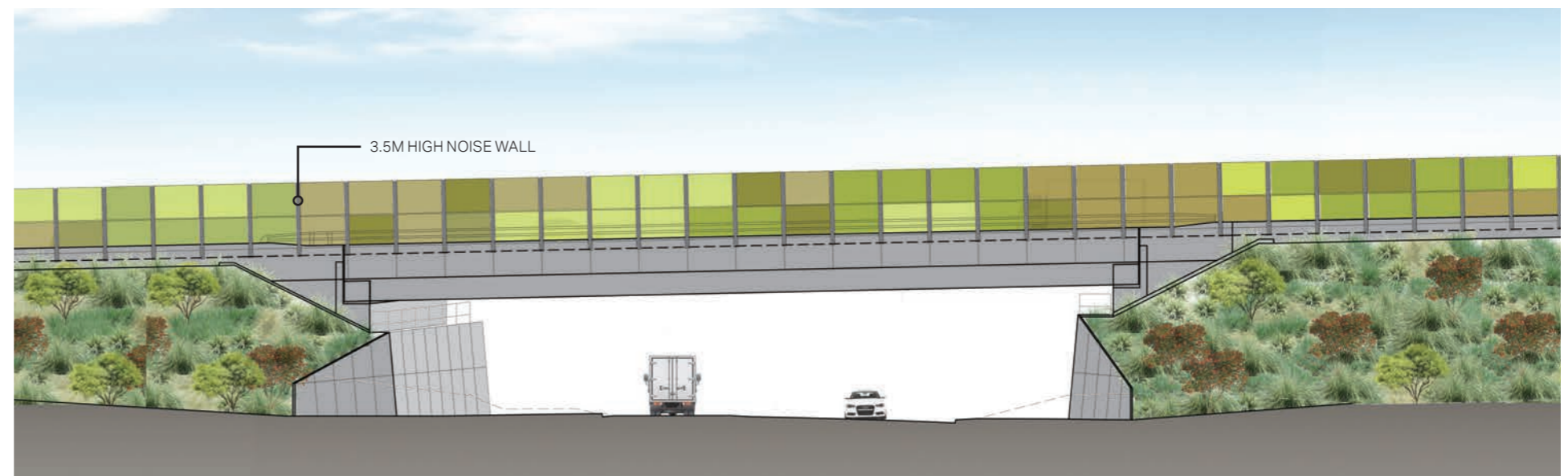
Figure 67: BR040 North Facing Elevation
