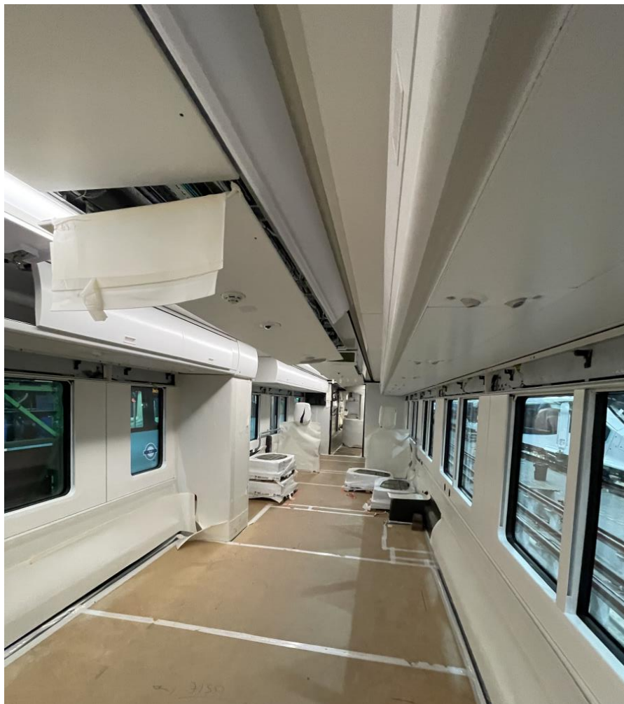
LR01 car following interior panel and fixture fit out
