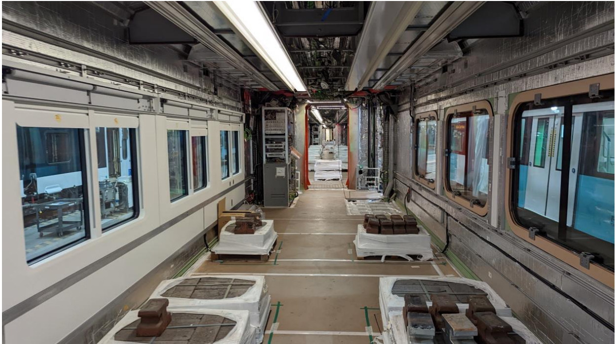
LR01 car being fitted out with interior panels and fixtures
