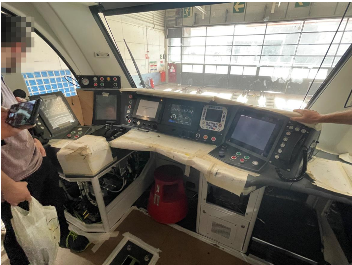
The crew workstation on LR01 undergoing modifications and testing
