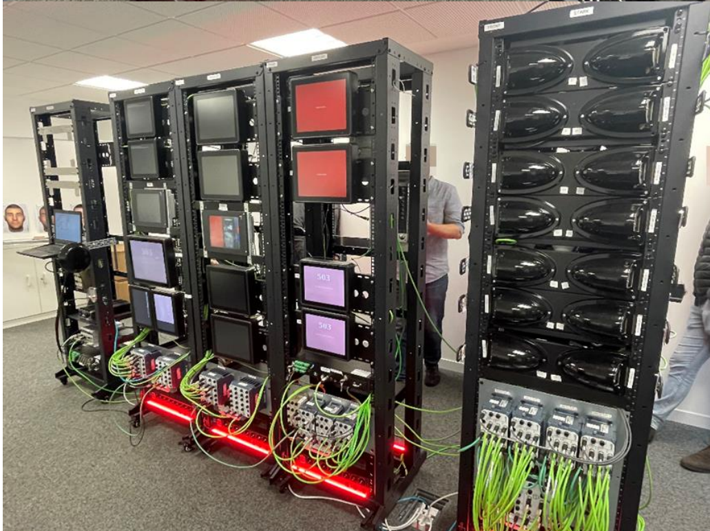
TfNSW and CAF reviewing the CCTV solution on the r2p test bench
