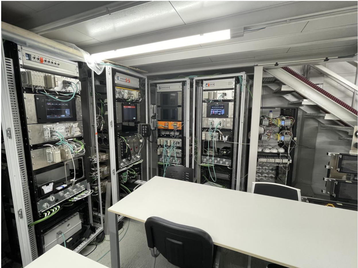
The CAF electronics test bench to simulate and test the on-board systems
