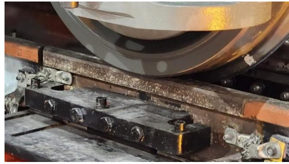
Weigh test load cell (closeup)
