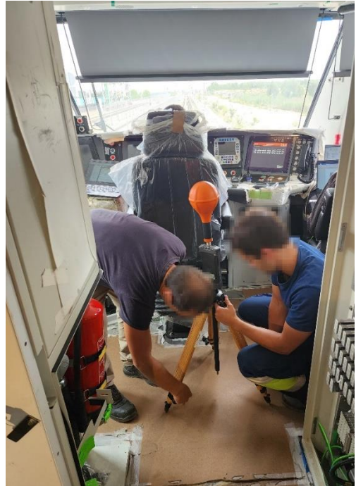
EMF emissions test in driver cab
