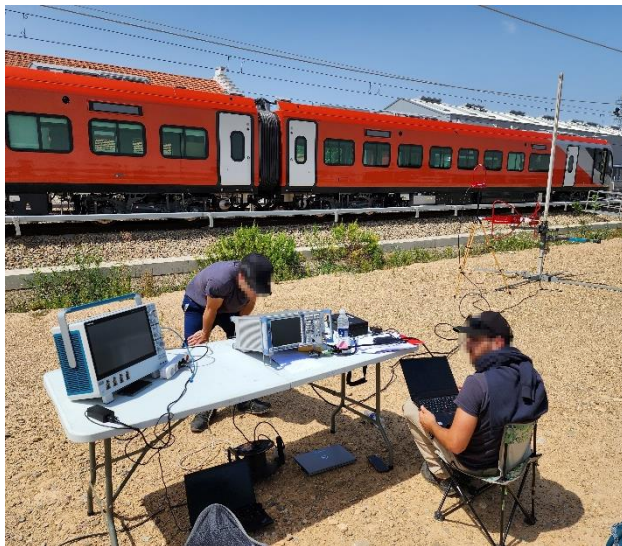
Preparing exterior test equipment for radiated emissions test
