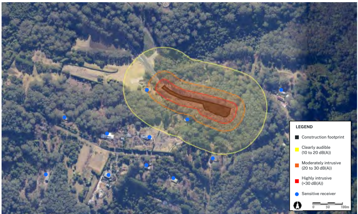
Figure 6-3: Potential daytime noise impacts - Slope 93282
