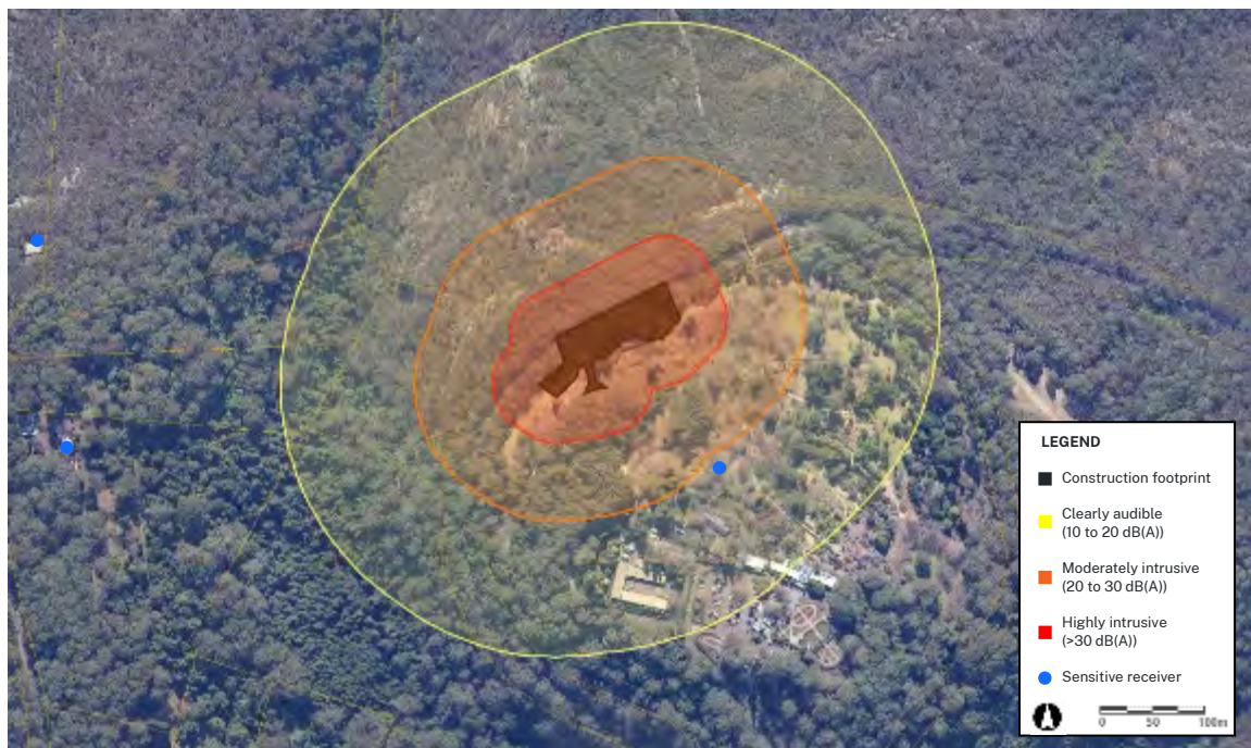
Figure 6-1: Potential daytime noise impacts - Slope 33459
