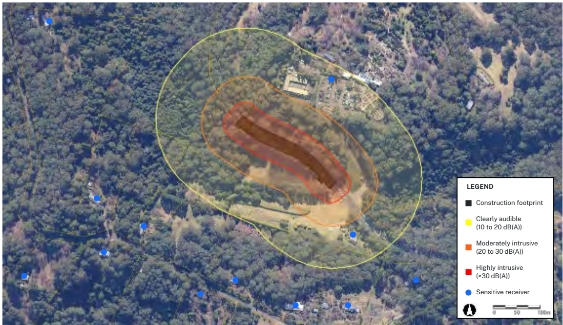
Figure 6-2: Potential daytime noise impacts - Slope 96403
