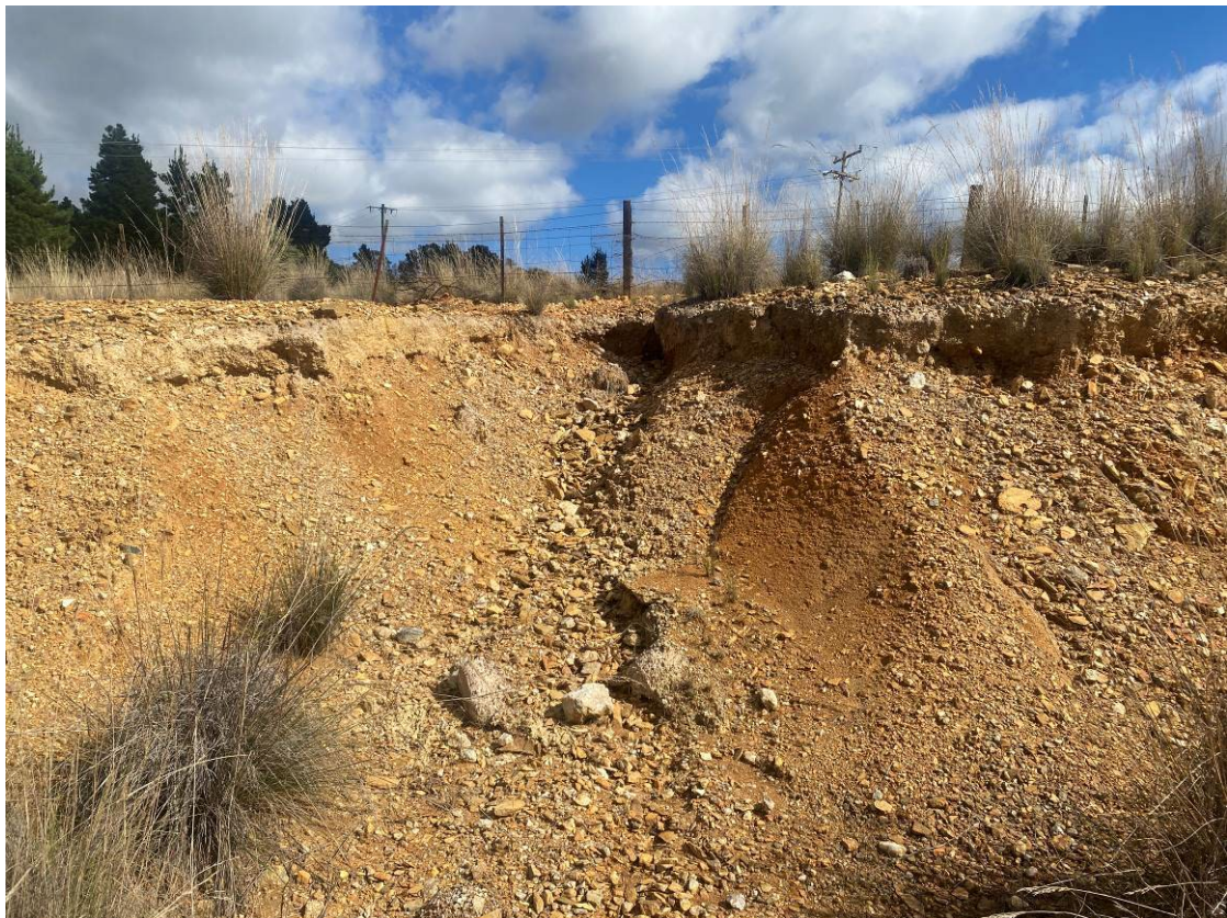
Photo 3: Evidence of erosion of soils on site. No evidence of current surface water runoff into Coppers Creek.
