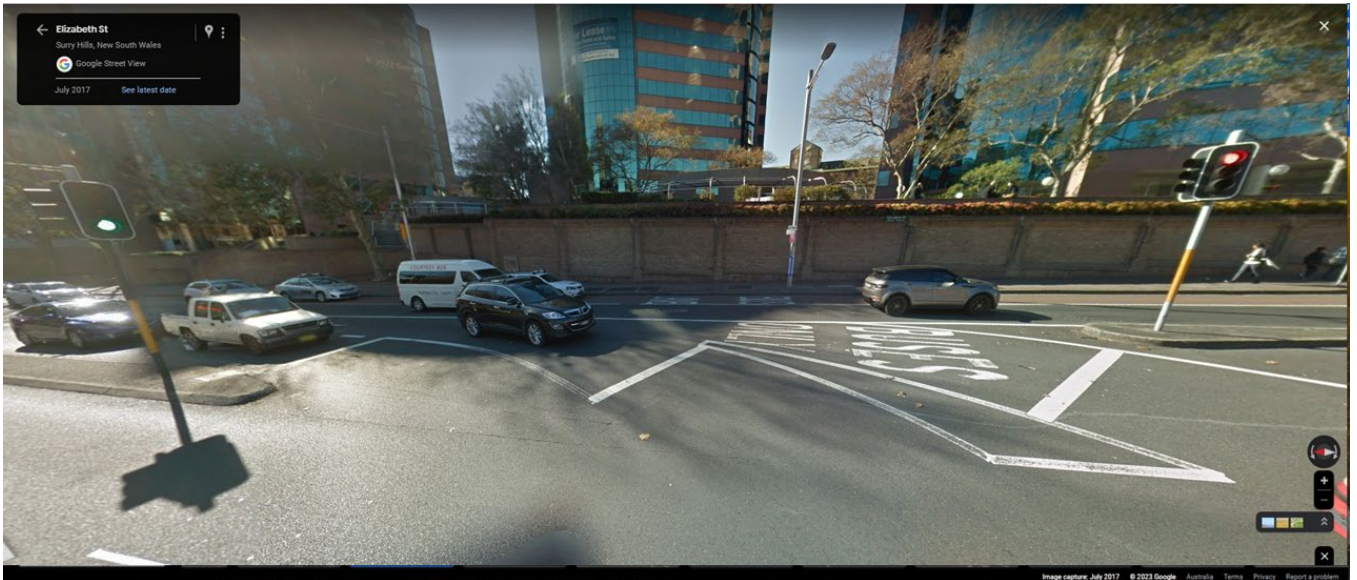
Figure 1. Example of continuous transverse lines representing staggered stop lines at a signalised intersection. In this example the continuous transverse lines delineate each lane separately.
