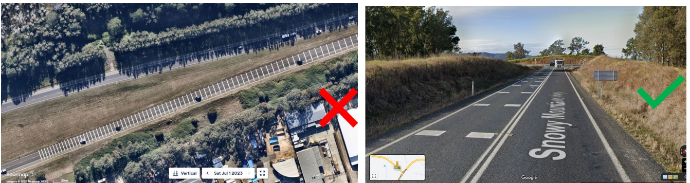
Figure 3. Examples of incorrectly and correctly applied line marking in a non-urban road environment.
