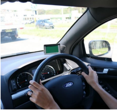
Figure 4 Example set up of display screen which provided alerts
