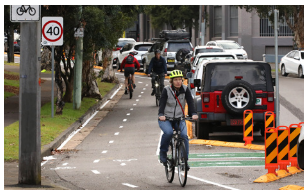
Figure 6.4 Pop-up cycleway facilities, like this one on Henderson Road, can be constructed quickly and with limited or no permanent changes to the road surface (Credit: Transport for NSW)
