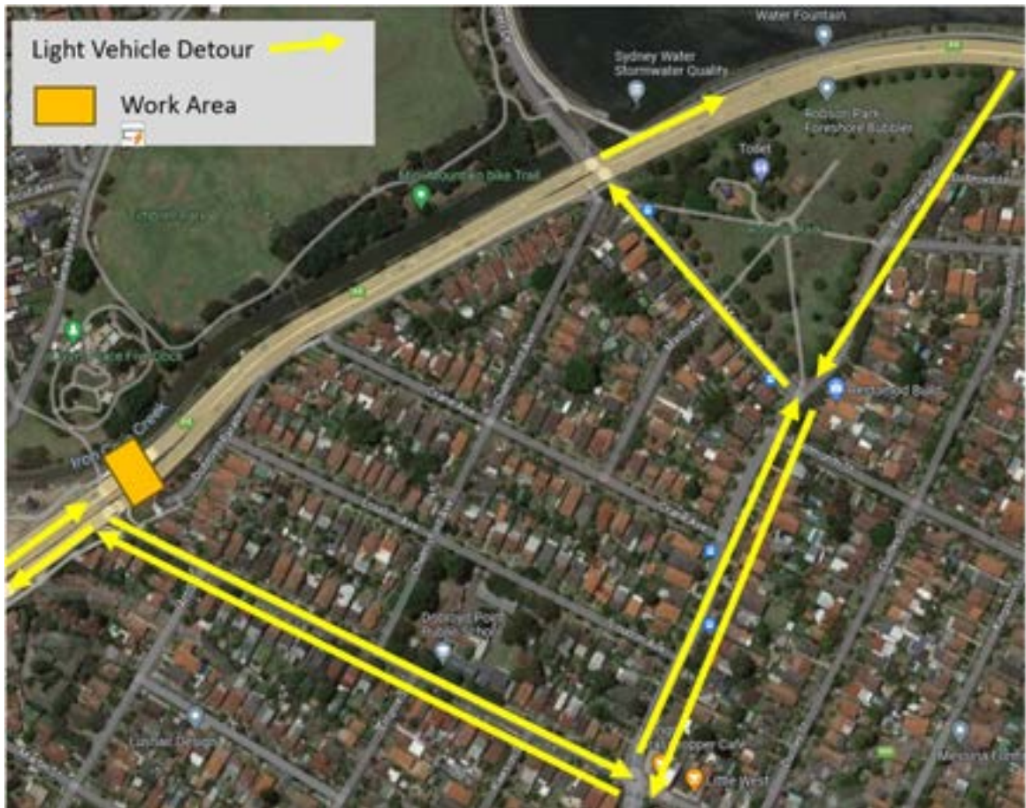
Figure 3-3 Light vehicle detour route
