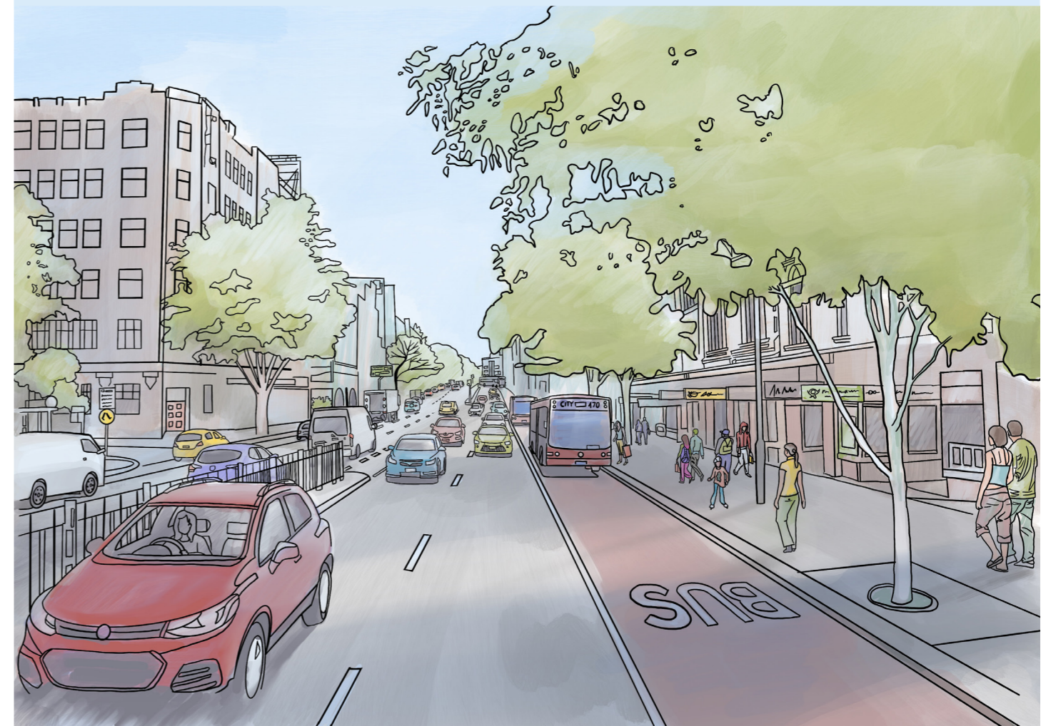
Example of reallocating traffic lanes to provide wider footpaths and a dedicated bus lane.
