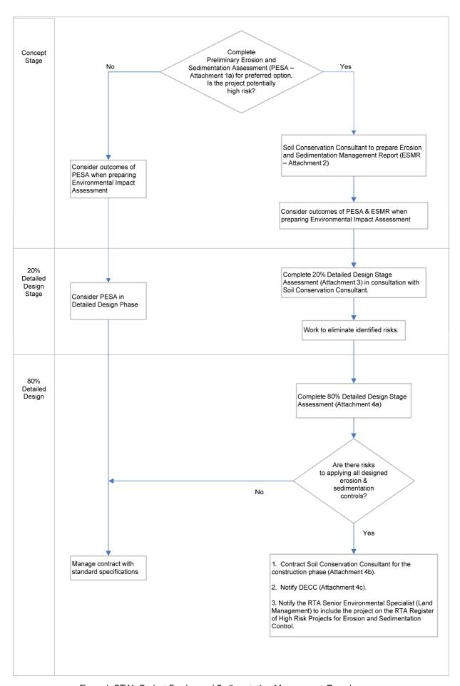
Figure 1: RTA's Project Erosion and Sedimentation Management Overview
