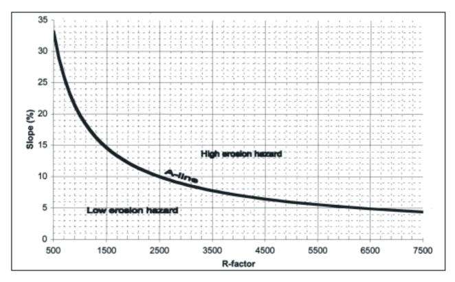
Figure 1b.1: Assessment of potential erosion hazard
