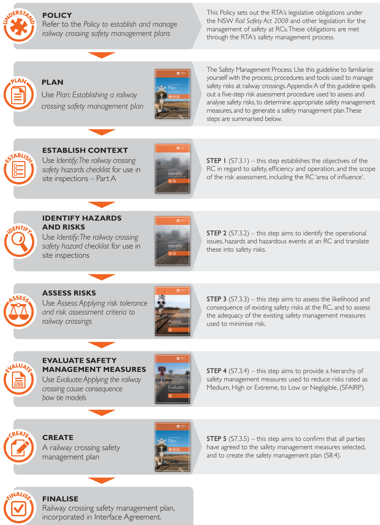
FIGURE 3: HOW DOCUMENTS AND STEPS RELATE IN THE ASSESSMENT AND MANAGEMENT OF SAFETY RISKS AT RAILWAY CROSSINGS
