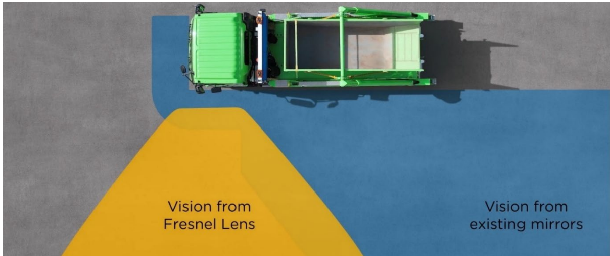
Figure 1 Fresnel lens field of view compared to traditional mirrors
