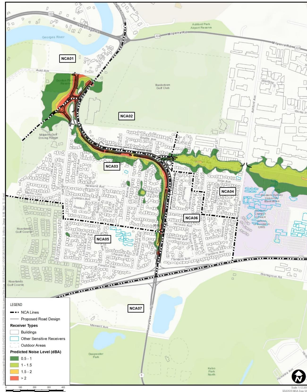
**Figure 15 Predicted Change in Road Traffic Noise Levels due to the Proposal**
