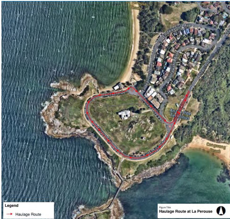
Figure 7-2 Haulage route at La Perouse
