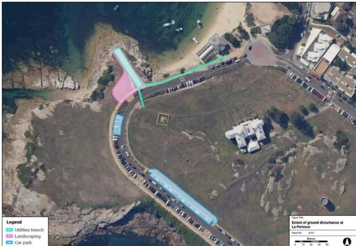
Figure 13 | Extent of ground disturbance at La Perouse during main construction (Source: EIS)
