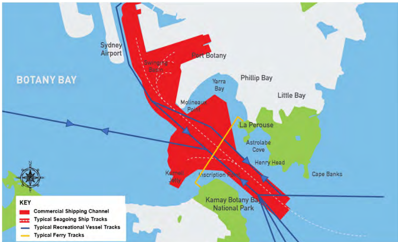
Figure 6-1 Typical passage of vessels in Botany Bay
