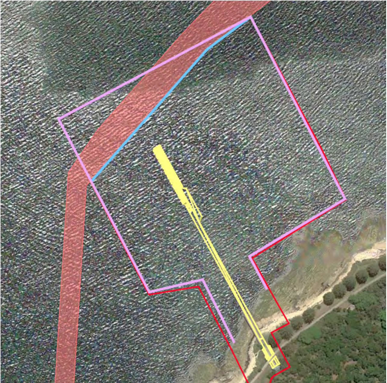
Figure 4-14 Proposed Marine Construction Zone at Kurnell
