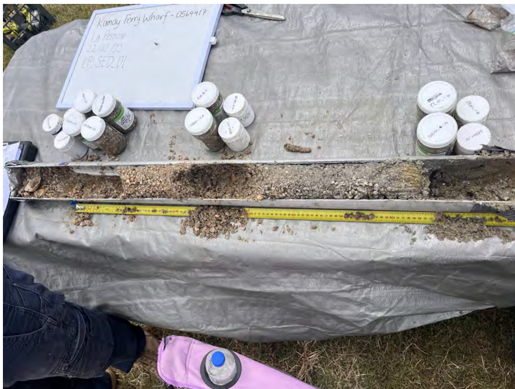
Figure 1: Sediment core being sub-sampled by Indiana Strachan from ERM
