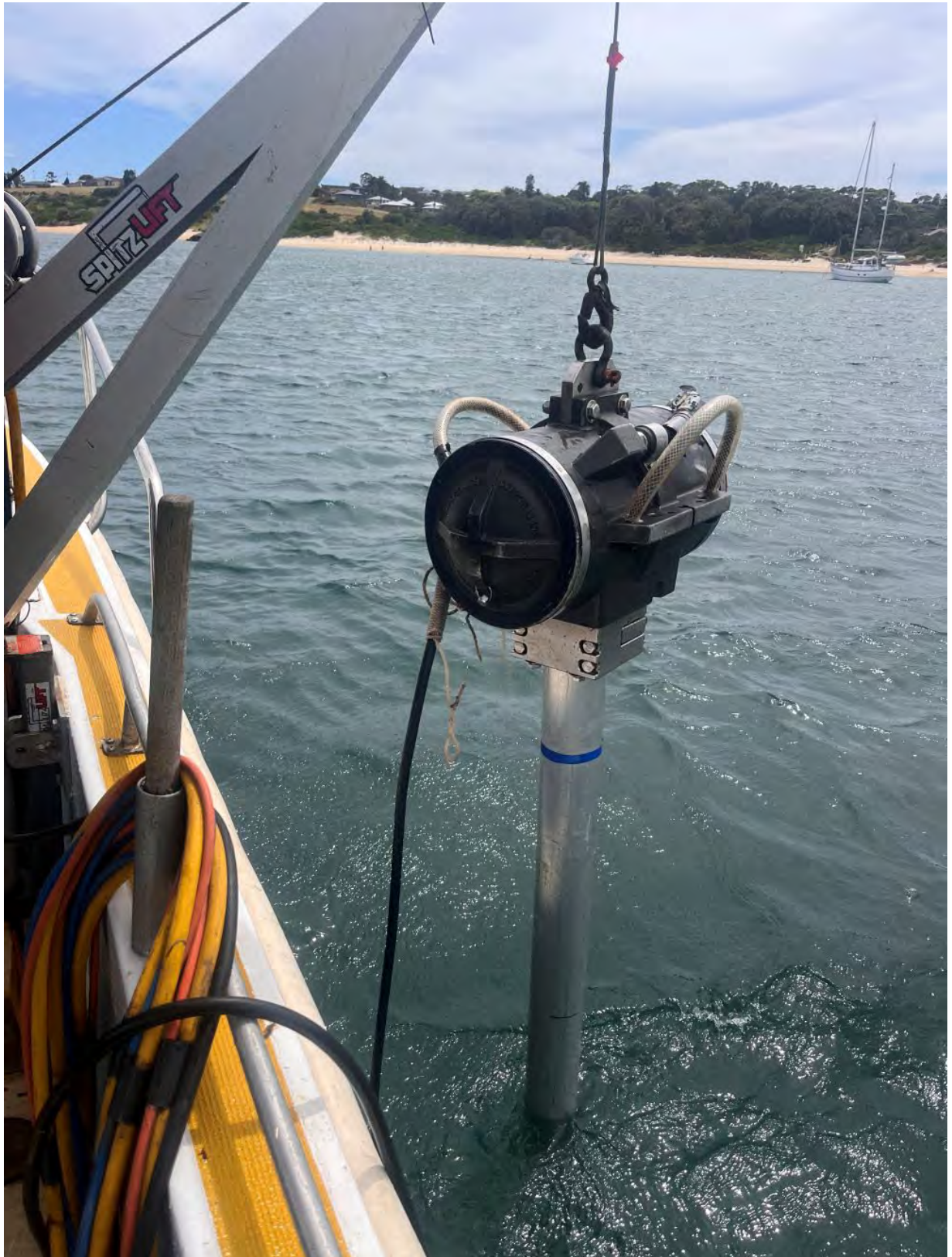
Figure 6: The vibrocorer with a core tube loaded ready to be winched to the seabed. The blue line on the tube indicates the one metre penetration mark.
