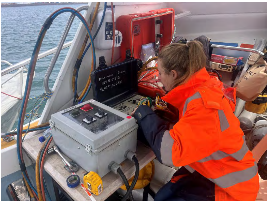
Figure 5: Diver Zoe Pocklington communicating with the diver, with the vibrocorer controls to her left, and breathing gas controls to her right.
