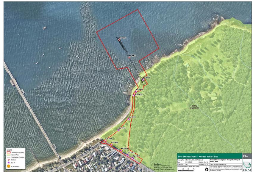
Figure D-2 Targeted Site Investigation – ACM Detections – Kurnell
