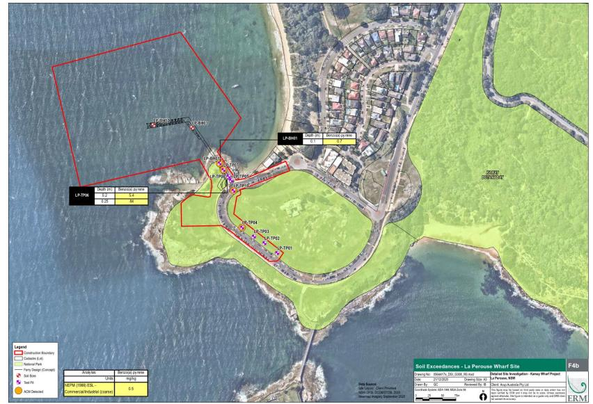
Figure D-1 Targeted Site Investigation – ACM Detections – La Perouse
