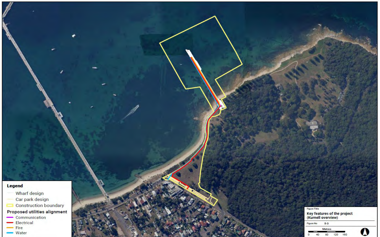
Figure 1-3: Construction boundary and key features - Kurnell
