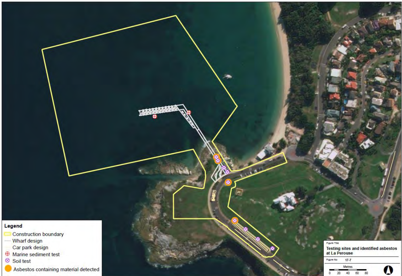
Figure 4-3 Identified Asbestos Containing Material (ACM) at La Perouse
