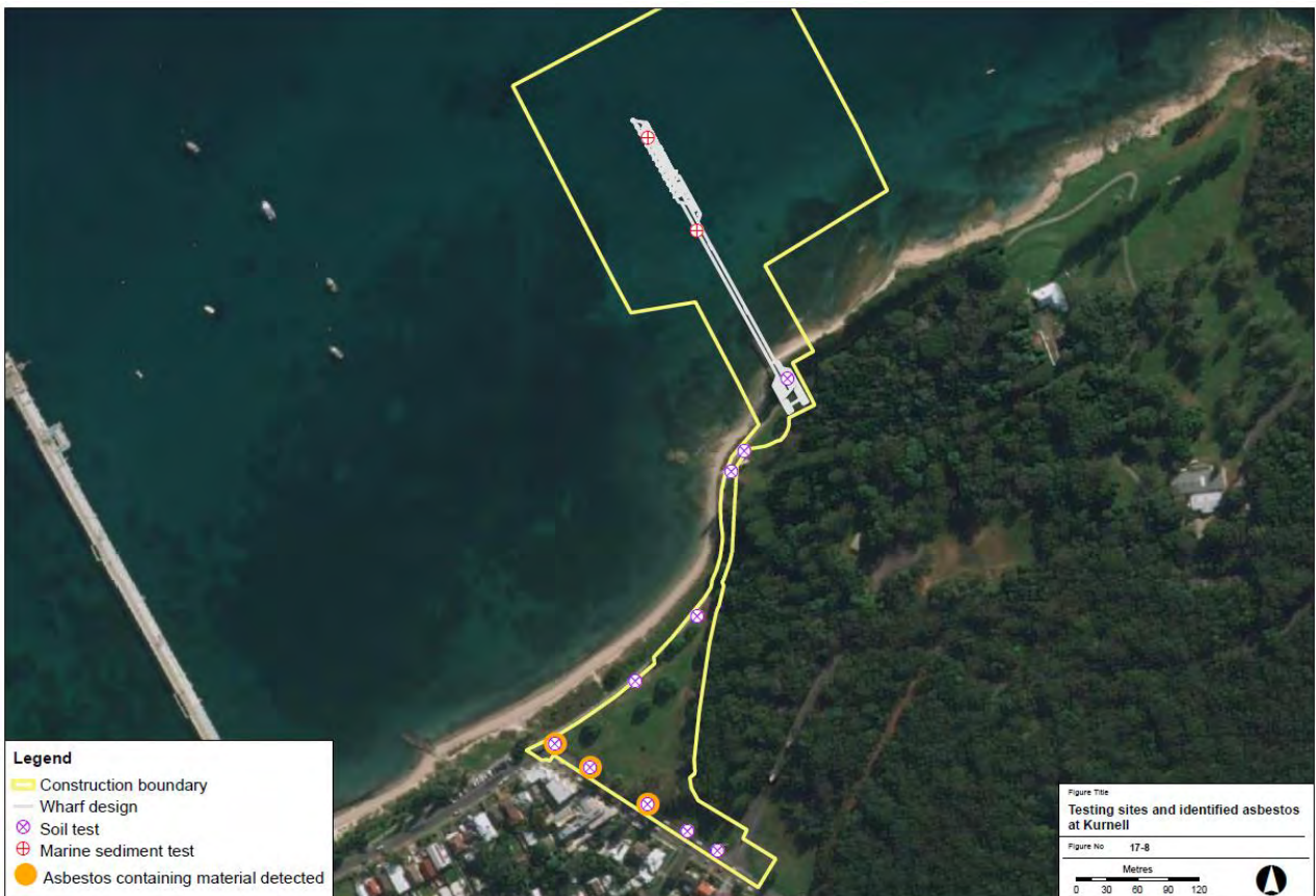
Figure 4-4 Identified Asbestos Containing Material (ACM) at Kurnell
