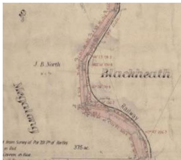
Plate 1: 1894 Plan showing areas proposed to be realigned. Note the square- corner as noted in the 1887 plan is proposed to be rounded off, as is accurate with the modern alignment (Source: LPI Crown Plan 1.2532)
