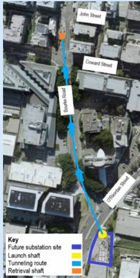
Map showing the underground tunnelling route
