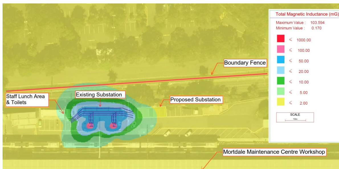
Figure 2 Existing Mortdale Maintenance Centre Substation – magnetic field contributions
