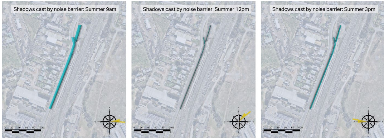
Figure 6-19 Shadows cast by the noise barrier along Lackey Road in Summer
