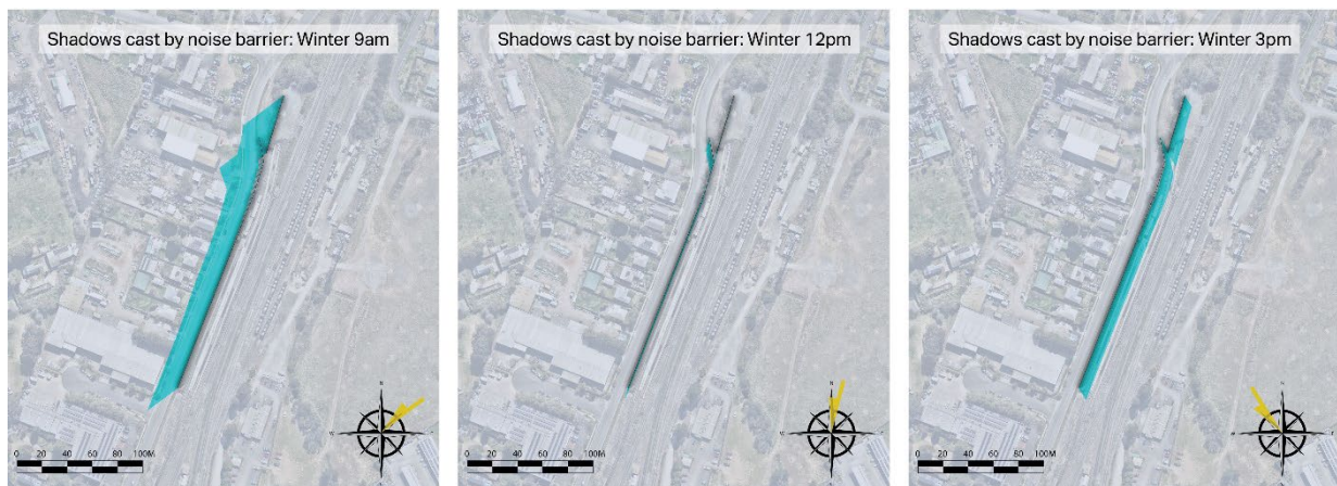
Figure 6-21 Shadows cast by the noise barrier along Lackey Road in Winter
