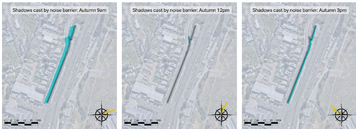
Figure 6-20 Shadows cast by the noise barrier along Lackey Road in Autumn
