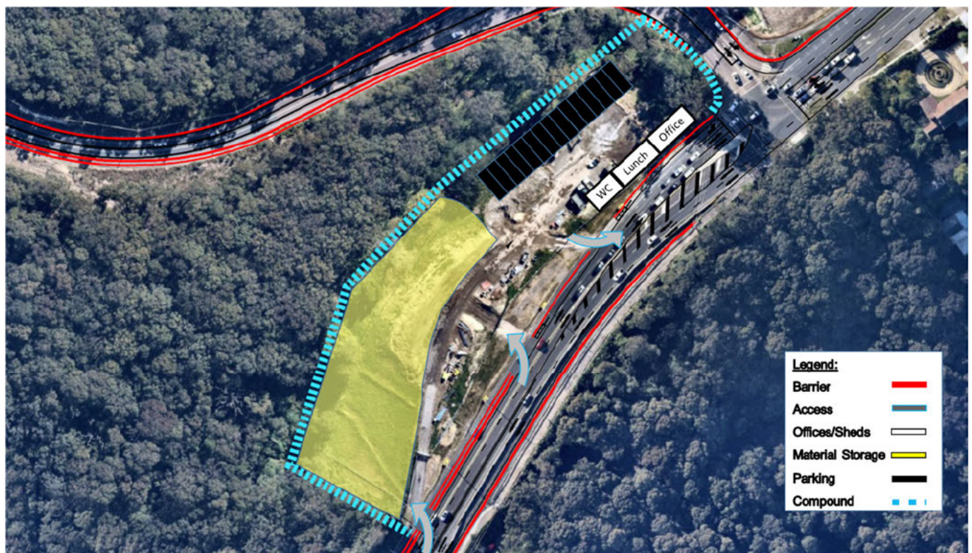
Figure 6: Construction compound F – Proposed Layout
