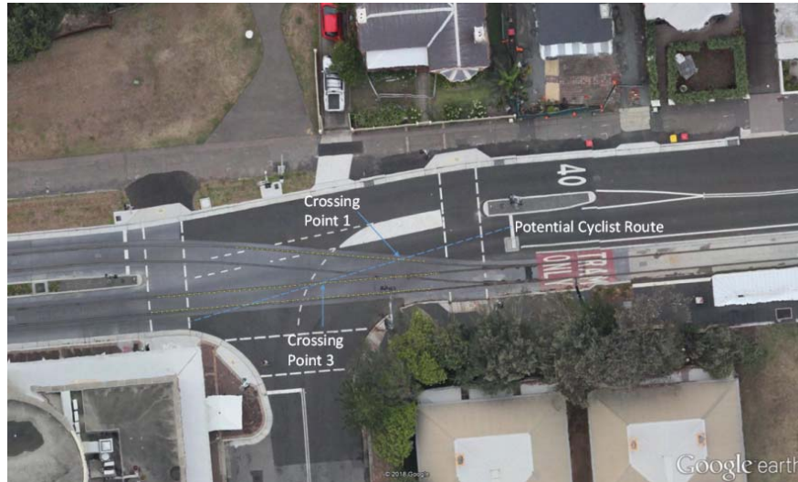
Calculation of cyclist crossing angles at eastern entry to mixed running section
