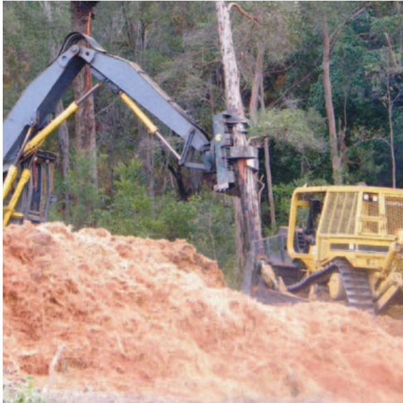
FIGURE 4.4: Tree removal using a claw extension to gently lower trees rather than dropping them. This machinery is suitable when removing habitat trees as it may reduce the impact on any fauna present inside the hollows (Photo: RTA).
