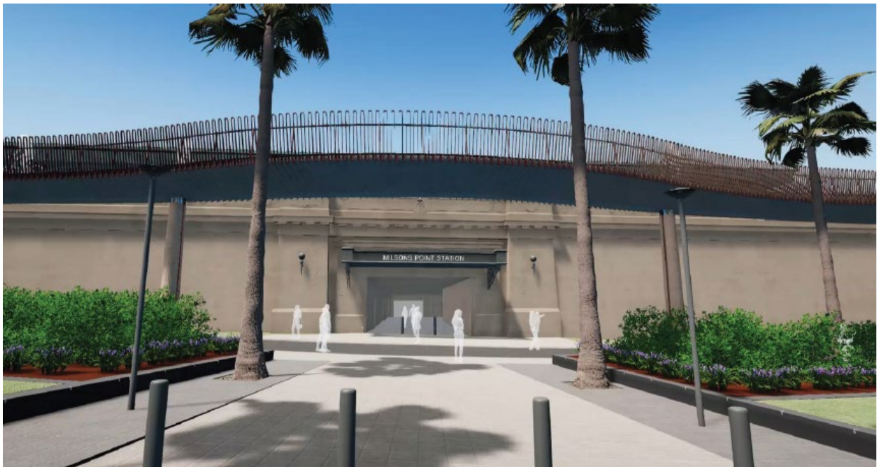
Figure 4-3: Design model view – view to the cartouche from the edge of the forecourt (note that the balustrade modelled shows the bronze finish) (model source: Aurecon)
