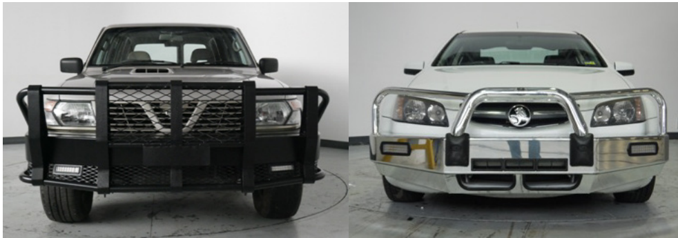
1.1 Heavy duty bull bar fitted to a 4WD
