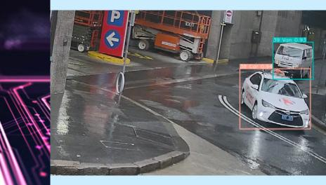
Transport has developed a cutting-edge computer vision prototype using Artificial Intelligence (AI) that successfully detects and matches vehicles entering and exiting freight facilities, carparks and loading docks.
