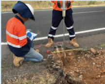
The strength of the subgrade (bottom layer of the pavement) is tested and measurements are recorded
