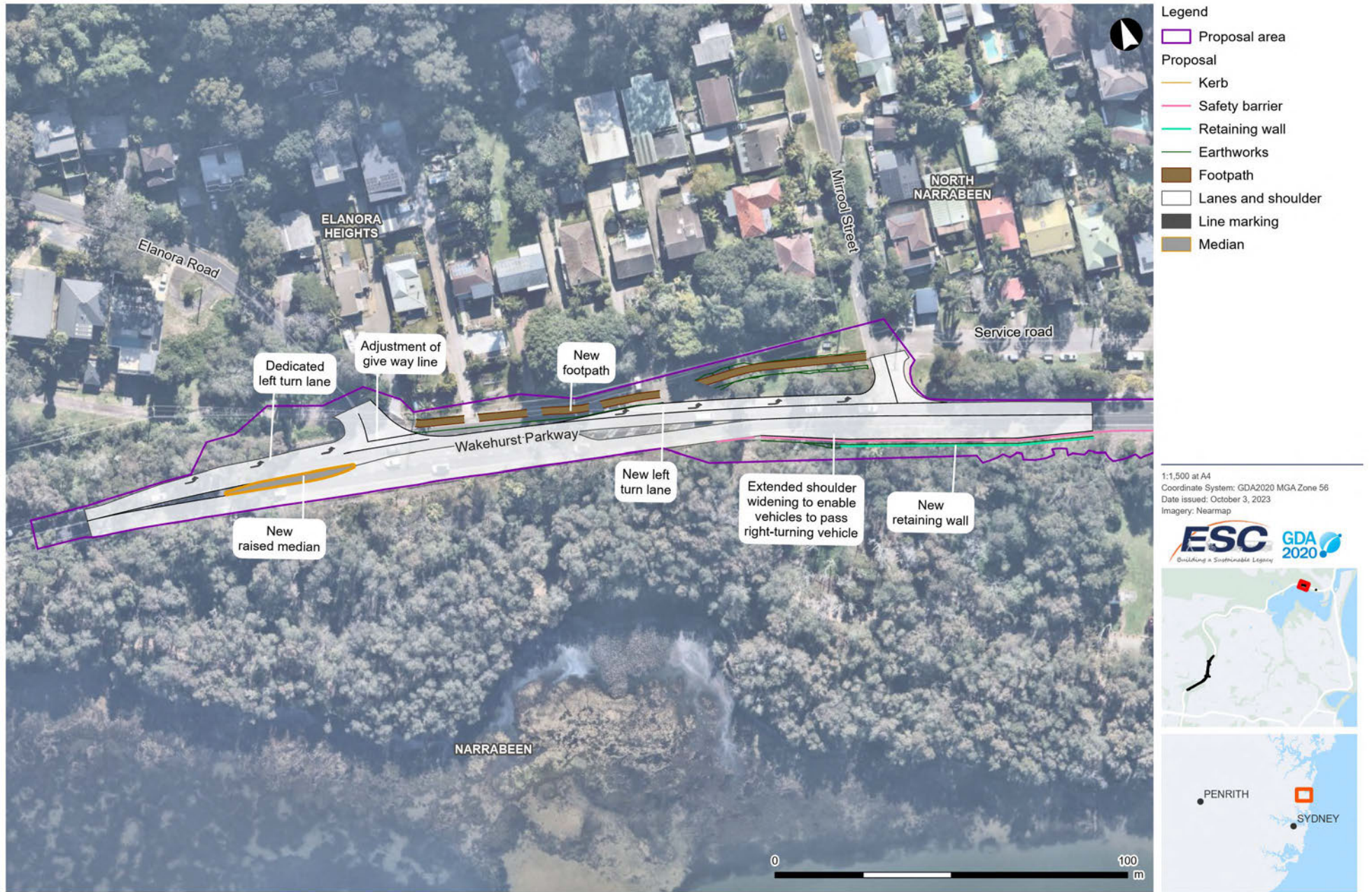
Figure 3-8, Key features of the proposal - Wakehurst Parkway from Elanora Road to Mirrool Street (Figure 1 of 3)
