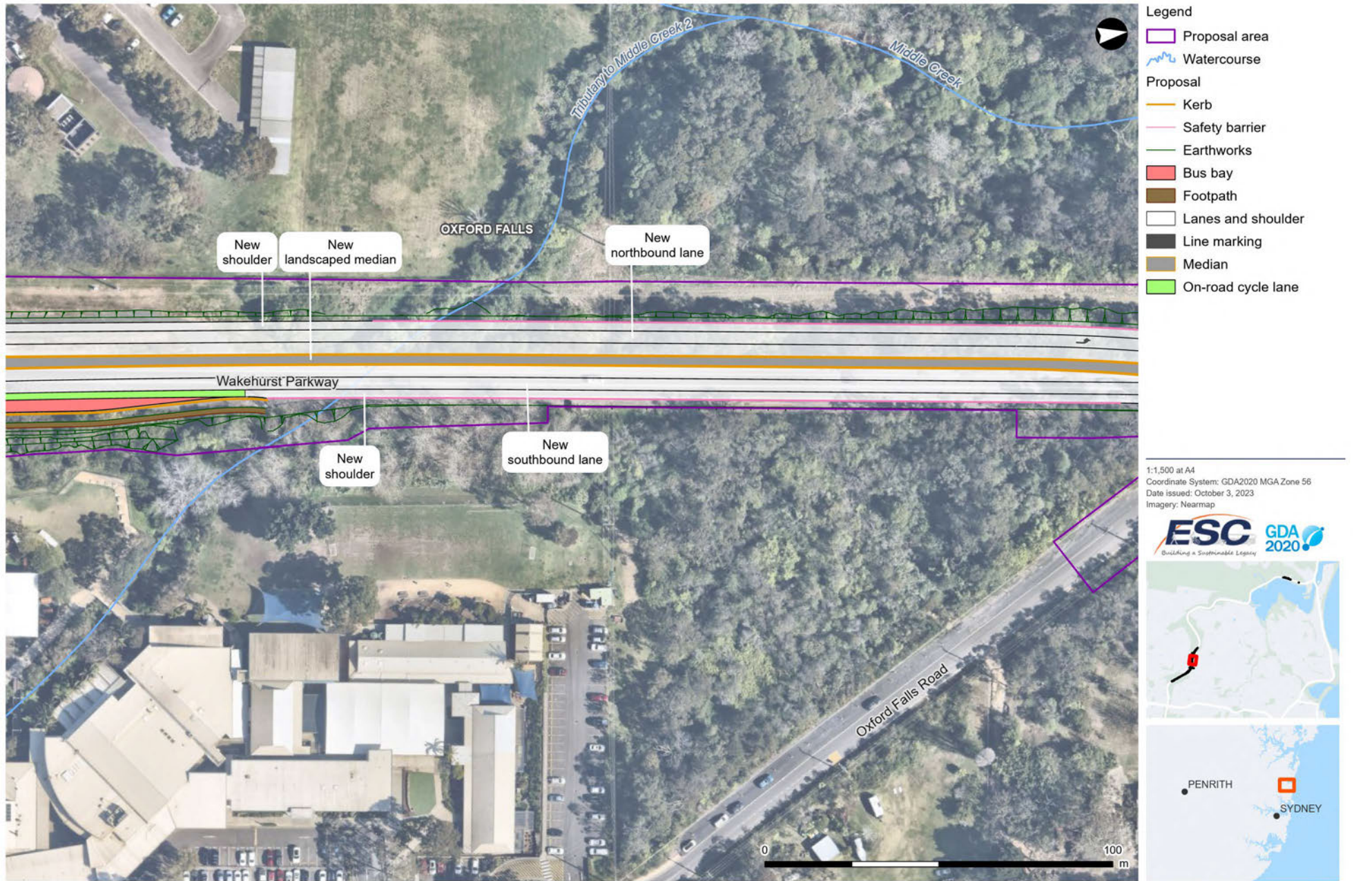
Figure 3-5, Key features of the proposal - Wakehurst Parkway from Dreadnought Road to Oxford Falls Road (Figure 2 of 4)
