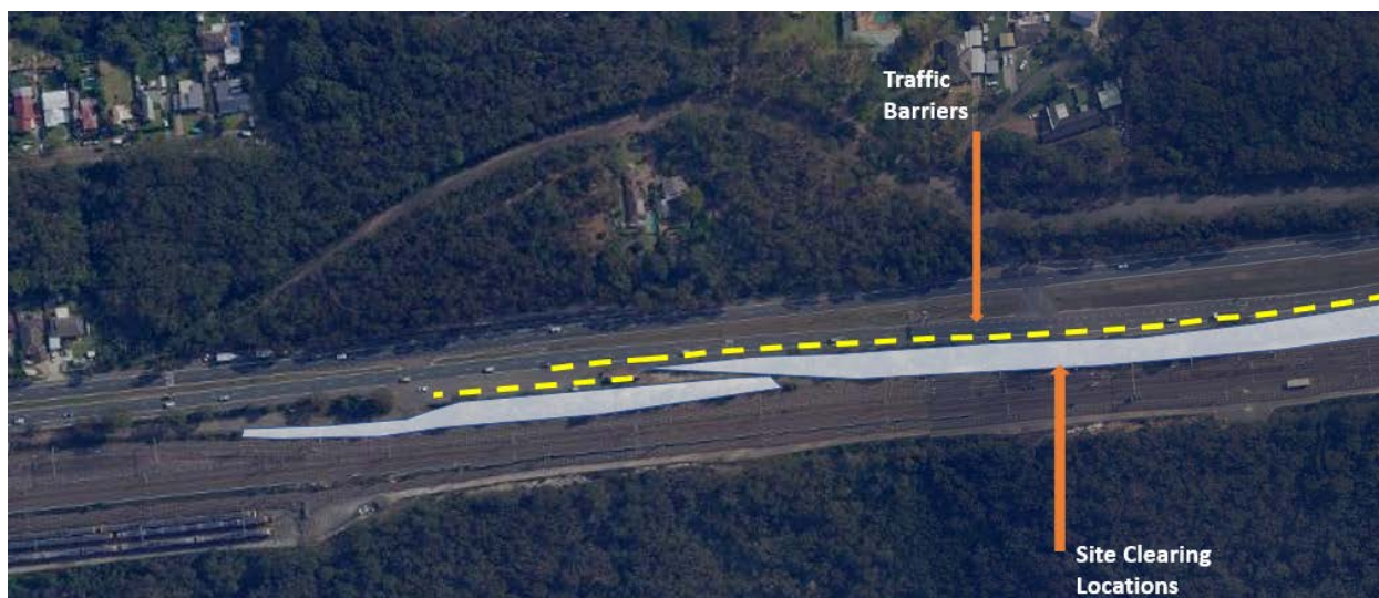
Image 2: Map showing location of installation of traffic barriers and site clearing on the Princes Highway near the truck stopping bay at Waterfall.
