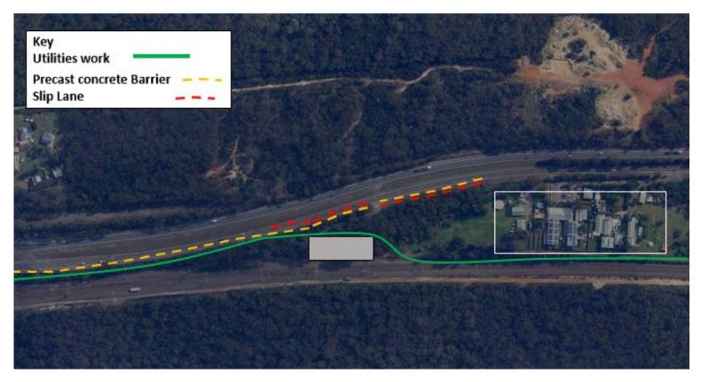
Image: Map showing location of the installation of traffic barriers and construction of the temporary slip road off the Princes Highway to allow for safe access to, and egress from, the site compound.
