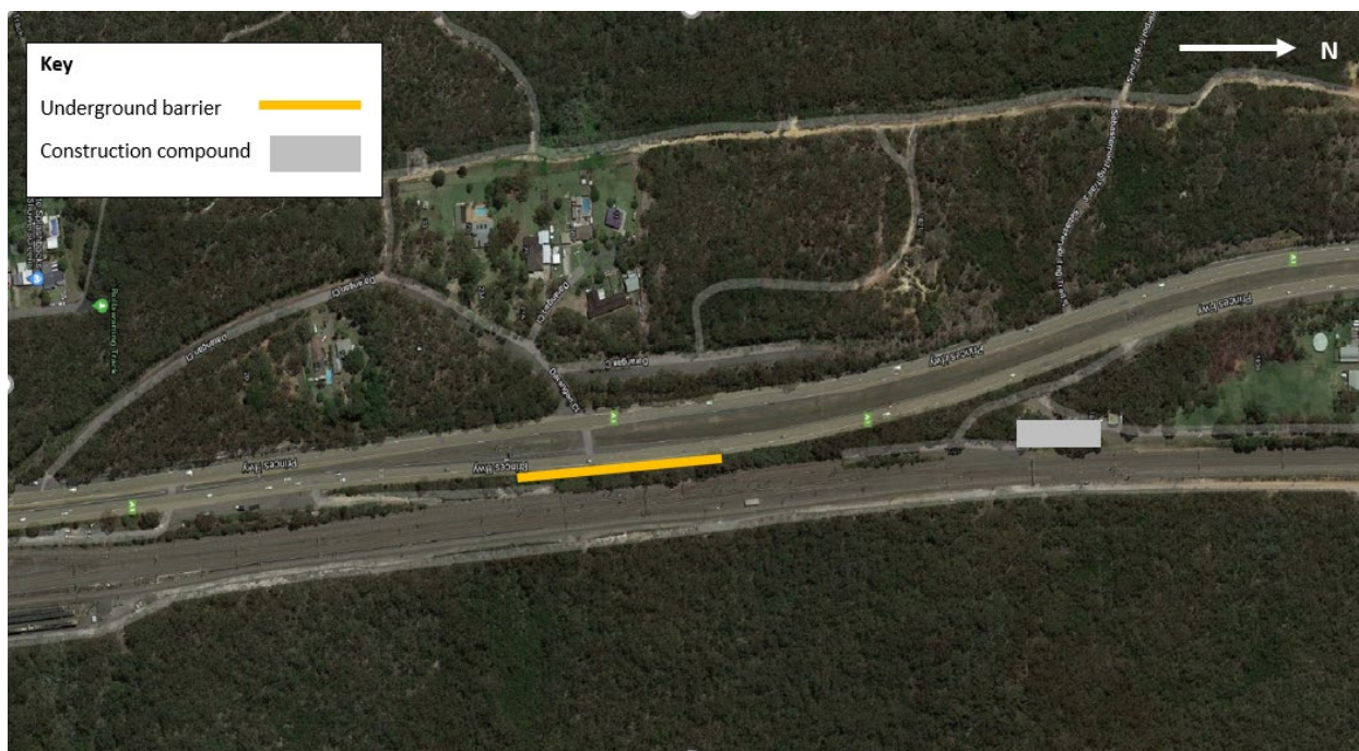
Image 1: Map showing location of work to install an underground barrier to protect utilities before piling work starts for the retaining wall.
