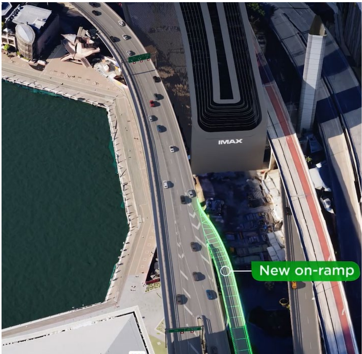
Figure 4-5: Representation of the solid line marking design alongside the Western Distributor merge from the Pyrmont Street and existing Fig Street on-ramps
